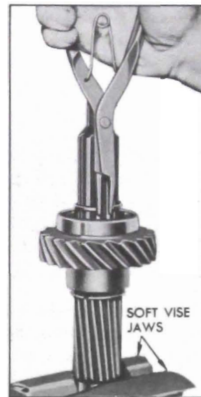
Figure 4-19—Removing Snap Ring from Main Shaft
